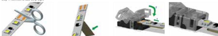
1-1: Cut LED Strip along the cuttable mark
